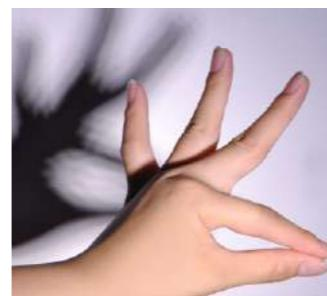
Fitting with single-LED-chip generates the lights from the scattered chips, making the subject blur and unclear in boundary with double image and consequently creating weak stereoscopic feel.
